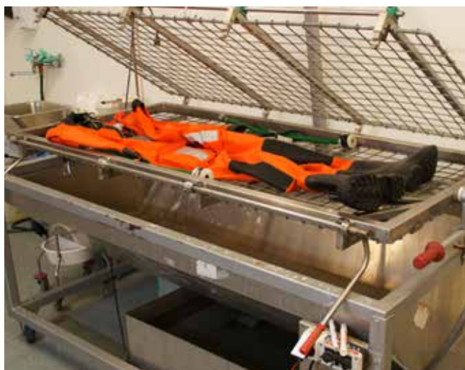
The drying cabinet is the most efficient way to prepare suits for delivery
