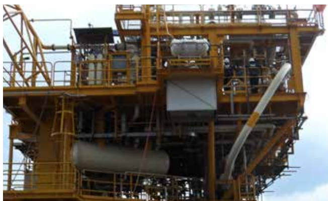
The container protects the evacuation chute against all types of weather
